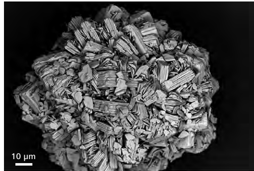
Lanthanum carbonate imaged at 1 kV with Inlens Duo BSE. \text{LaCO}_3 is a phosphate binder used as an oral therapeutic agent for dialysis patients.
