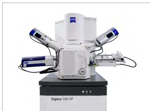
Gain information on topography and composition with Sigma 560 configured for throughput in analytics: two coplanar EDS detectors for information on chemical elements and an EBSD camera for crystallography.
